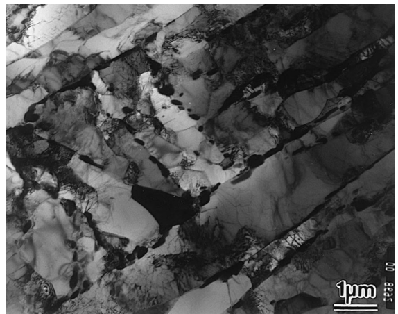
Fig. 2. Microstructures in an irradiated sample of about 3.4 dpa.
